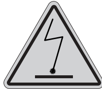
Electrostatic Discharge Hazard
