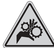
Pinch Point/ Entanglement Hazard
