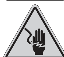
High Voltage Hazard
