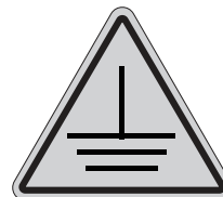
Grounding Required Hazard
